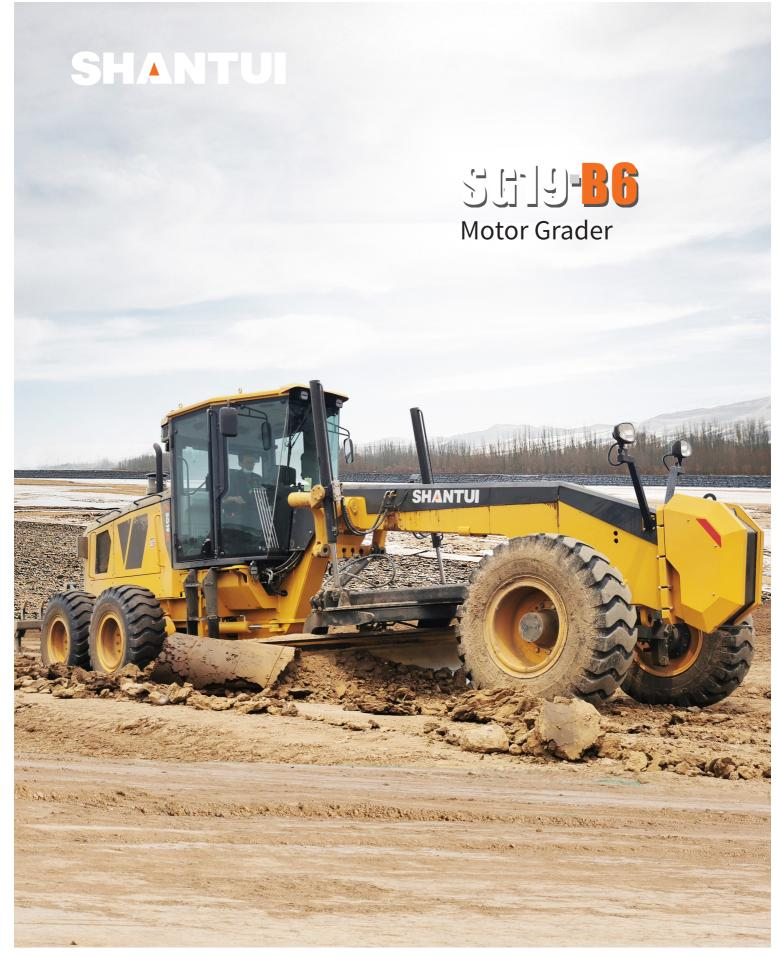
Engine Model: Gross Power: Operating Weight: Cummins 6CTAA5.9-C205 153kW @ 2200rpm 15,800kg We Level Subgrade Fast and Flat easy operation and maintenance
